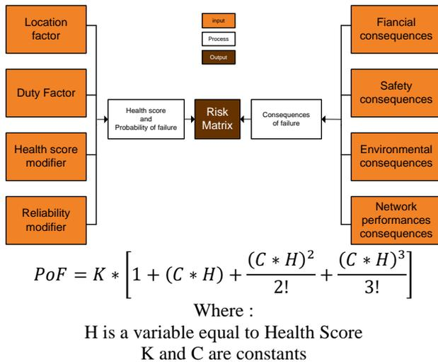
Figure 1 : CNAIM risk matrix calculation based on probability and consequences of failure
