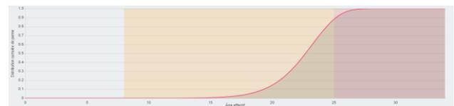
Figure 3 : Probability of failure for LV transformers of the example analysis
