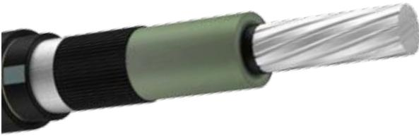
**Innovation.** Light and resistant, our Lo-Sag aluminum alloy aerial conductor with composite core significantly increases line transmission capacity and overload. It operates at up to 180°C and expands 10 times less than a conventional conductor. As a result, it delivers the same level of security with lower pylons at greater intervals (spans of up to 2.5 km).
