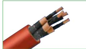
Available in light, flexible and compact rubber versions for large turbines (2.5–8 MW), these 1-, 3-, or 4-core cables can withstand three full twists in either direction. These cables can use standard connectors, and therefore save time and money.
