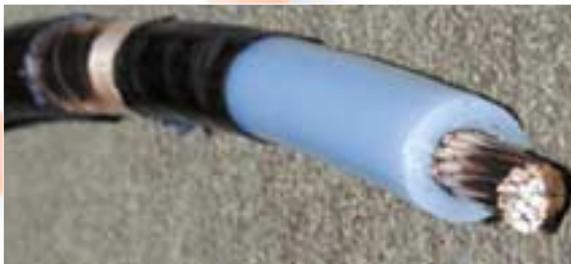
Prototype extruded cable
