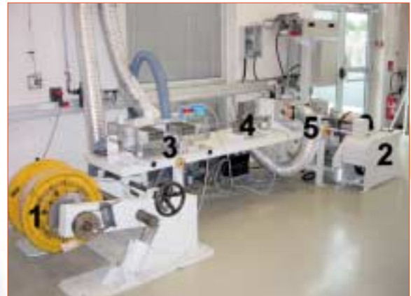
Figure 2: cable pilot coating line set up in the R&D lab pay-off / take-up stations, corona treater, coating chamber and UV-curing lamp.
